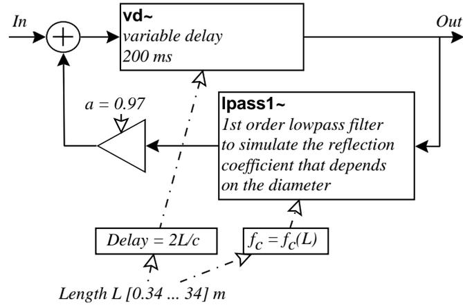
Figure 20: Implementation of the basic shape "Cylinder".
