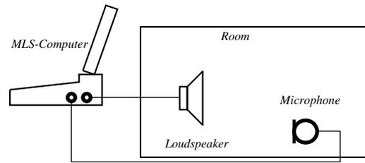
Figure 17: Experimental setup for room impulse measurements.
