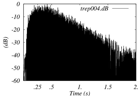
Figure 10: Echogram of a staircase.
