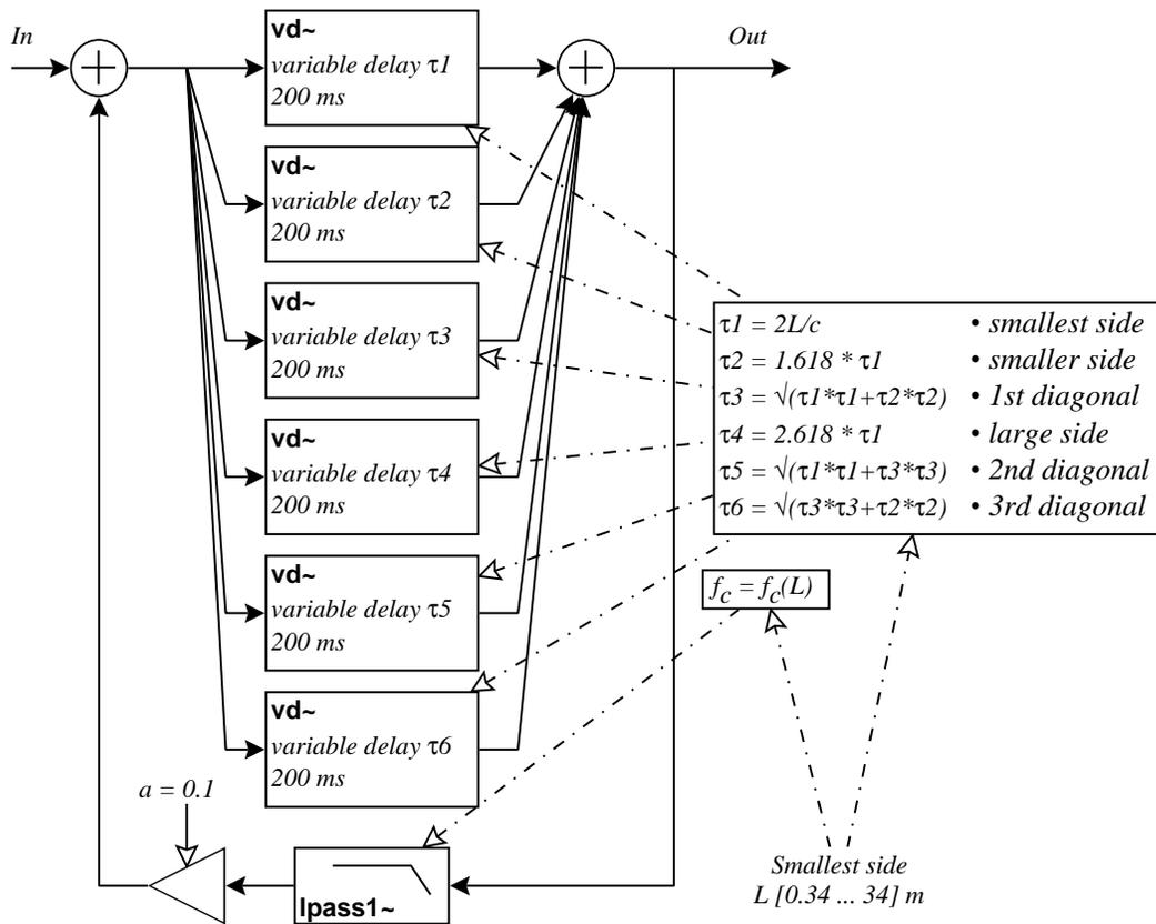
Figure 21: Implementation of the basic shape "Parallelepiped".
