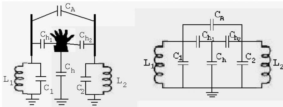
Figure 3. The equivalent electrical scheme in our application.
