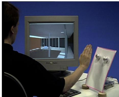
Figure 2. Setup of the system of EFSs for navigation in virtual environments.
